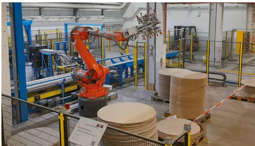
Papeteries de Clairefontaine - robot for the automatic laying of cardboard discs
